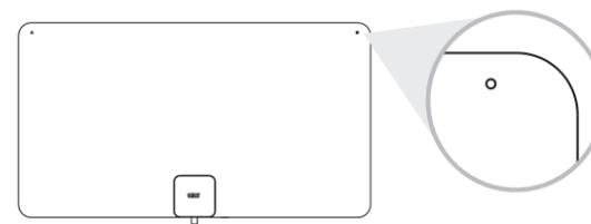
Insert two of the included push pins into the two holes on the top of the antenna.
