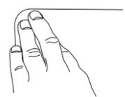
Line up the antenna and press it against the mounting surface for 10 seconds. Let go, then press 30 seconds more.
