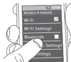
Make sure the **PAIR** indicator on the front of the speaker is blinking rapidly. (If it isn't, give a short double-press on the **⏻** button. The speaker gives an audio signal.)
