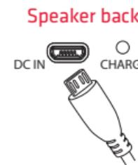
The **CHARGE** indicator on the back of the speaker is red while the speaker is charging. It turns off when the speaker is fully charged.
