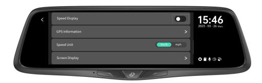
Speed Display: Choose if the vehicle speed is embedded into the DVR video files.
