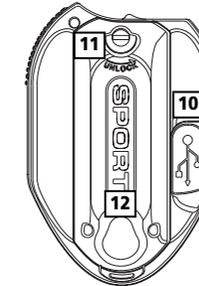
10. **USB port** (🔌) - Attach the small end of the mini-USB cable here.
