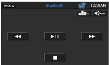
Bluetooth provides an Advanced Audio Distribution Profile (A2DP) profile for streaming music from a wireless phone or a Portable Multimedia Player (PMP), sometimes referred to as a MP3 player. The unit allows you to play back audio files from your wireless phone or a PMP using a Bluetooth connection. Before using an audio player, it may be necessary to enter the default passkey into the unit. The default passkey for the unit is "1234".
