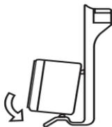
3. The Sound Bar will snap into place on the Sound Bar Bracket.
