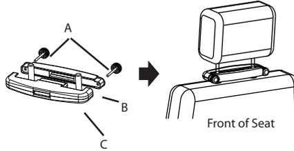
4. Secure the brackets in place with the Screws. Turn the Screws clockwise and hand tighten.
