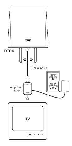
The amplifier insert connects directly to the back of your TV via the built-in cable connector.
