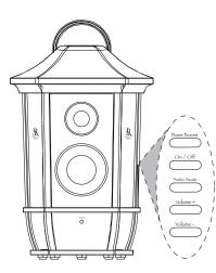
1. Press the Power button on the side of the speaker to turn it on.
