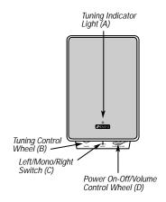
**Note:** Interference in the form of static and/or distortion can sometimes be heard. If this occurs, confirm the transmitter/speaker adjustments and indicators. If the problem persists, refer to the **TROUBLESHOOTING** section of this manual.
