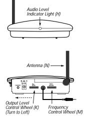
**Note:** If the light does not flicker, confirm secure connection of the AC Adapter. If the light still does not flicker, confirm secure connection to the audio source **output**. If there is still no response, leave the Output Level Control Wheel completely to the left (as shown) and see the following **Note**.
