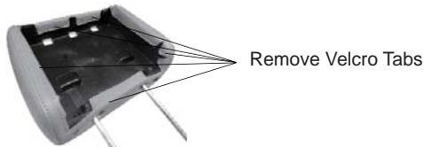
3. Replace the headrest cover with the black or pewter cover and secure the headrest cover by re-attaching the velcro tabs.
