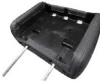
4. Pull the monitor cables back out of the tubes while lowering the monitor into position. Hook the tabs at the top of the monitor into the top of the headrest and align the two holes in the monitor with the screw holes in the headrest.
