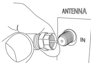
Make sure your TV is turned off. Then connect the amplifier's coaxial cable to the antenna input on your TV or digital converter box.
