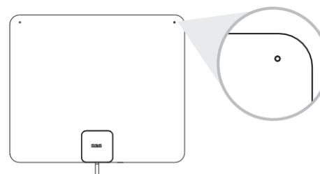
Insert two thumbtacks (not included) into the two holes on the top of the antenna.
