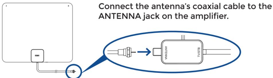
Connect the antenna's coaxial cable to the ANTENNA jack on the amplifier.
