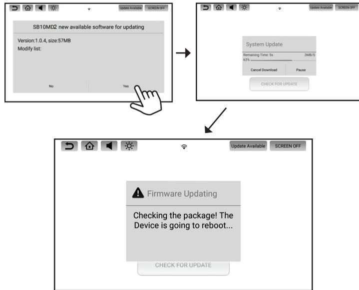
**NOTES:** Do not disconnect power from the monitor during the update process. Once the software download is complete, the system will check the downloaded files and then begin the update process. When the update process is complete, the monitor will return to the standby mode. Press the Power Button to turn the monitor on and resume operation.
