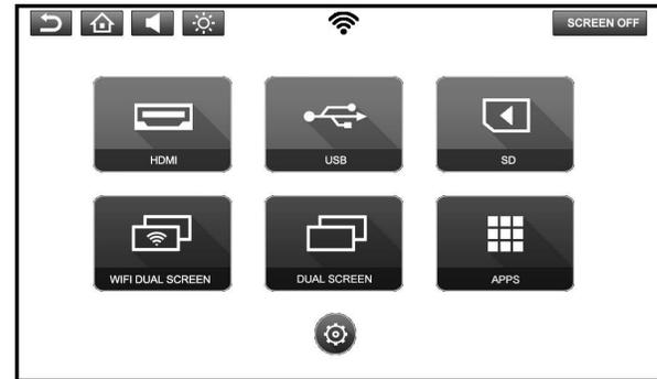
2. To stop mirroring content on the receiving monitor, press the Home button on the receiving monitor.
