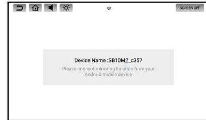
4. After a few seconds, the Receiving monitor's Device Name will be displayed under "Available Device" on the Transmitting Monitor.
