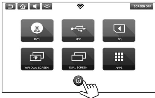
2. Select "ABOUT DEVICE" in the SETUP screen, touch the "CHECK FOR UPDATE" button to check for new software availability.
