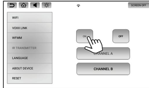
4. Select the desired Channel (A or B) for the IR Transmitter. It is recommended to select Channel A for one monitor and Channel B for the other monitor.
