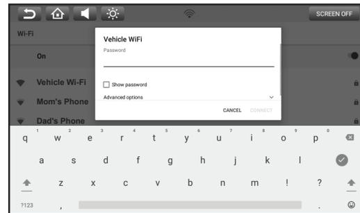
5. The monitor will now connect to the Wi-Fi network. Once a Wi-Fi network is saved into memory, the monitors will automatically reconnect to that network as long as the Wi-Fi setting is set to "ON".
