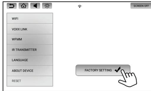
**NOTE:** The RESET function deletes all user settings, any installed APPS, and reverts the system monitors back to their factory default state. The RESET buttons on the side of each monitor resets the system monitors without deleting user settings.
