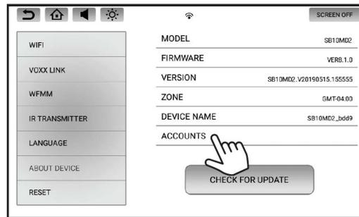
2. Tap "ACCOUNTS" to access the stored account information on the monitor. Tap the account you wish to remove, then press "REMOVE ACCOUNT" to remove/delete it from the monitor.
