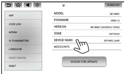
2. Tap "DEVICE NAME" three times to display the keyboard. When you are finished renaming the monitor, press "OK" to save the new monitor name into memory. Renaming the monitor allows you to uniquely identify it on the network when using the Voxx Link APP. Refer to page 18 for more details.
