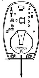
Carefully remove the discharged battery by sliding it out from under the clip in the direction indicated by the arrow in the diagram. Properly dispose of the exhausted battery and insert a new CR2032 taking care to arrange it so that the + is facing up toward the + symbol on the battery clip. Reassemble in the reverse of above.
