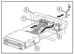
CAUTION! The rear of the radio must be supported with the strap to prevent damage to the dashboard from the weight of the radio or improper operation due to vibration.
