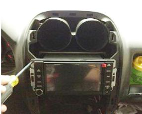
7. Plug in all supplied harnesses included in kit make sure CAN module is properly connected 8. Mount the radio with the 4 OEM Philips bolts.
