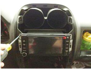
5. Unplug radio harnesses and remove factory
