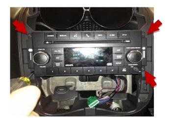
4. Remove 4 Philips head bolts securing the radio
