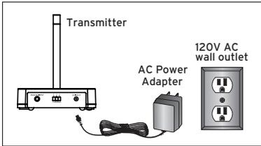
Connect the small, round plug from the transmitter AC power adapter to the transmitter's power input jack. Plug the other end of the transmitter AC power adapter into any standard 120V AC wall outlet.
