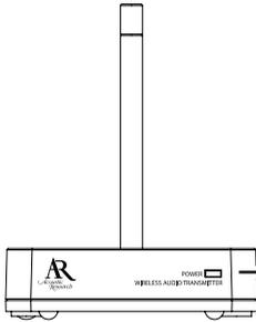
**POWER indicator** lights blue when audio is present and the transmitter is broadcasting
