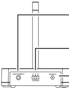
**Built-in audio input cable** connects to your sound source using one of the connection options shown on the next pages
