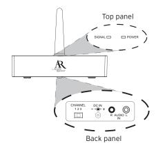
**SIGNAL** indicator lights green when the audio is present and the transmitter is broadcasting **POWER** indicator lights when the transmitter is on CHANNEL 1 2 3 lets you find the best transmission frequency for your environment **DC IN** jack receives the small round end of the included 12V 200mA AC power adapter AUDIO IN (R / L) connects to your sound source using one of the connection options shown on the next pages
