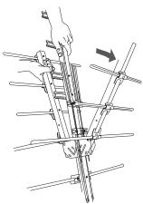
Once you've unfolded all of the elements on the reflector booms, extend the reflector booms away from the main boom until they lock into place.
