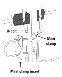
Find the U-bolt and mast clamp insert (see the illustration to the left). Put the U-bolt into the mast clamp insert with the teeth of the mast clamp insert facing the closed end of the U-bolt.
