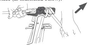
Turn the middle section over and unfold the shorter elements on the other side.
