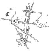
Each reflector boom has four elements. Unfold each slightly. Then, starting with the element closest to the main boom, unfold the element until it locks into place.
