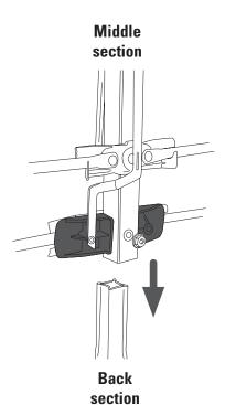
On the middle section (the one you unfolded in step 2), find the word "Back" stamped in blue on the boom. Find the same stamp on the boom of the back section. Line up both booms so that the stamps face you.
