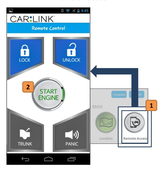
Once properly set up, you are able to use your application to access your remote start kit\* by pressing the 'Remote Access' button [1]. From here you can start/stop your vehicle, lock/unlock the doors, pop your trunk, activate panic siren or even access auxiliary options\* [2].
